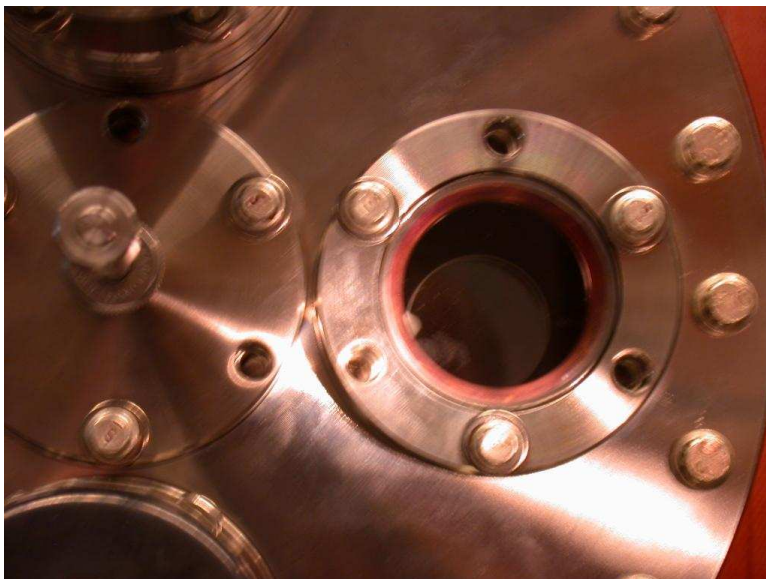
Fig. 35.— Photo of the “lollipop” device installed in the machine; the sapphire window is visible through the glass. SXR is connected to the flange just visible at the top of the image—in order to block it with the sapphire lens, all we had to do was rotate the shaft counterclockwise.
