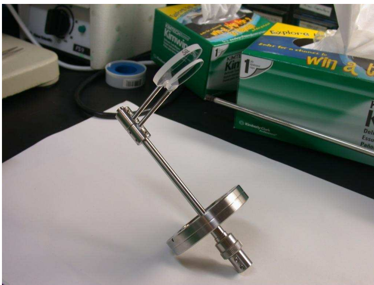
Fig. 33.— SXR “lollipop” device. The large window is made of UV-fused silica (transmission cuts off abruptly above 7.3 eV, and the small window is sapphire (transmission cuts off above 8.3 eV). Once the device was installed in the machine, the windows were oriented at 90 degrees with respect to one another. Rotating the device then allowed us to position either window in the SXR line of sight.
