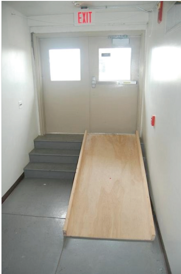
Figure A1. The ramp was constructed of sturdy 19-mm plywood, reinforced with wooden beams to safely afford locomotion. It was mounted on steps, as shown, but surrounded on three sides by black felt curtains to avoid providing any relative orientation information. The rear curtain was made to be irregularly shaped and was bunched at the bottom where it contacted the ramp to avoid the formation of a dihedral angle. Participants initially stood at the base and were asked to look at a dark red fixation mark in the middle of the ramp while making a verbal judgment. They then stepped onto the ramp and made a second verbal judgment based on haptic perception. They could not see the surroundings.
